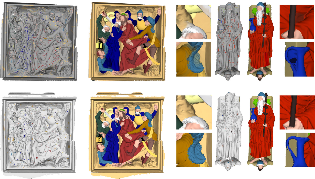
Fig. 2 Comparison of the colorization results of [44] ( first row ) with the one of our approaches ( second row ). Our method considers directly the raw point cloud and does not require any preprocessing, whereas
